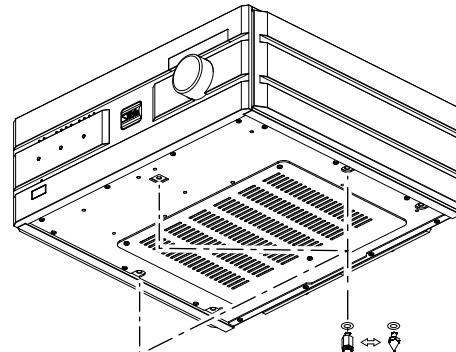
The feet can also be attached to the back-side holes. If the front side of the device is not stable, attach the feet to the back-side holes.
