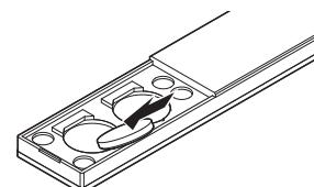
5. Insert the claw on the rear cover into the slit and then close the lid.
