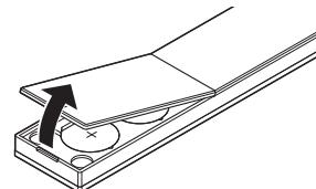
3. Use a thin yet sturdy oblong object to remove the batteries. Do not use any metal objects.
