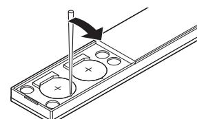
4. Insert the batteries with the + side facing upwards from the side indicated by the arrow.
